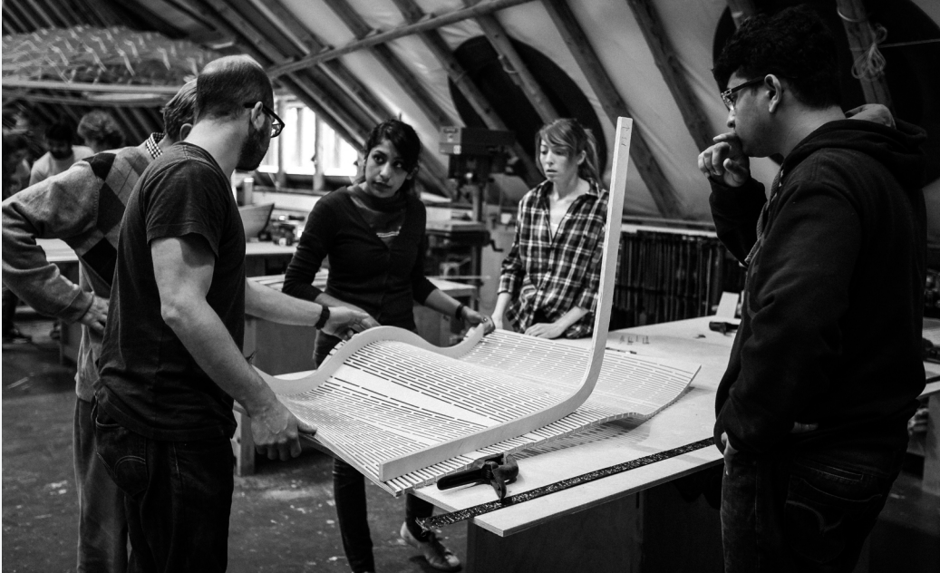
▲ Figure 1 Students and staff testing the use of a jig while prototyping a high-curvature panel of Carbon Curve. Credit: AA Emergent Technologies and Design
