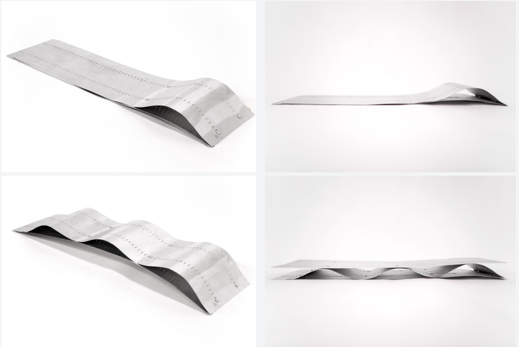
▲ Figure 12: Waterjet cut and digitally predetermined configurations.
