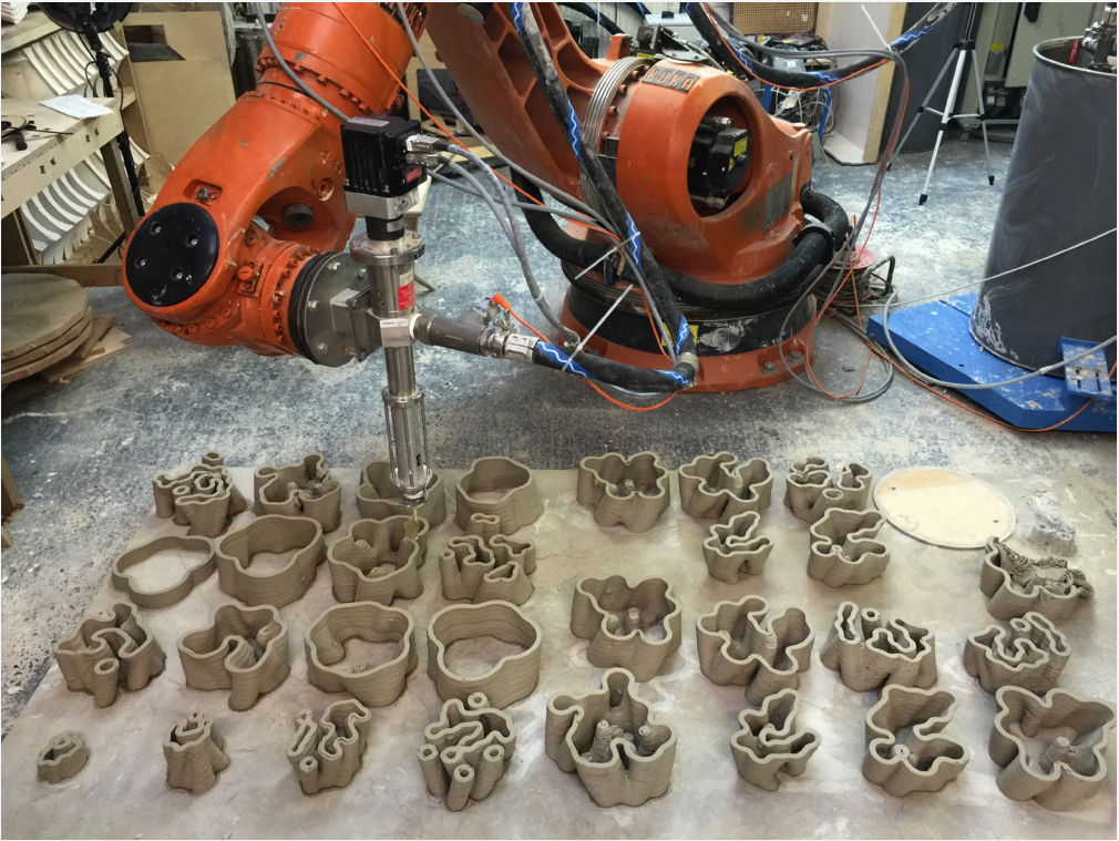
▲ Figure 1 Robotic arm extruding multiple segments of clay objects. Photo credit: Guan Lee.
