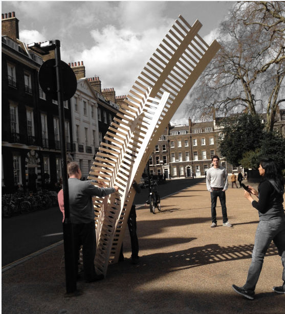
▲ Figure 2 Early prototype of a portion of the catenary arch testing tolerances and friction connection between elements in Fingers Crossed. Credit: AA Emergent Technologies and Design.
