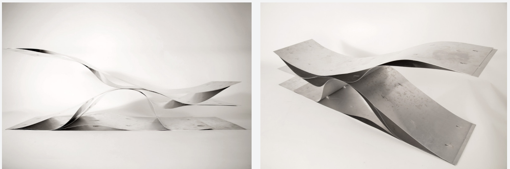
▲ Figure 13: Dynamic changes in layer hierarchies, waterjet cut and assembled without material deformation (material stays within the elastic range of deformation).
